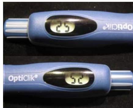
Figure 2. If held upside down when dialing a dose of 25 units (top), the actual dose selected is 52 units (bottom).
